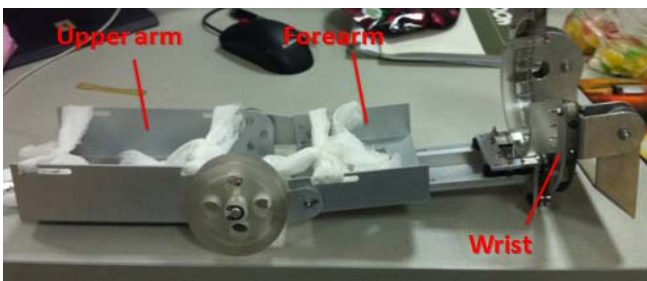
Fig. 2 The prototype of the upper limb exoskeleton rehabilitation device
