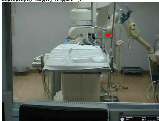
Fig6 Surgery scene of remote surgery (red arrow show Mechanical arm, black arrow show auxiliary part.)
