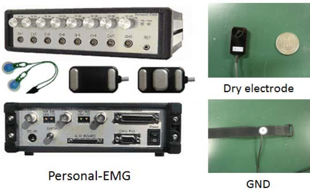
Fig2. Experimental setup of sEMG acquisition
