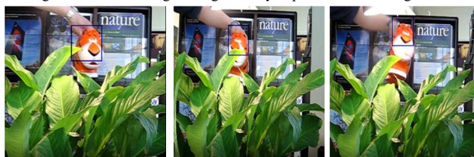
Fig.8 The result of target recognition by Camshift algorithm with Kalman filter.
